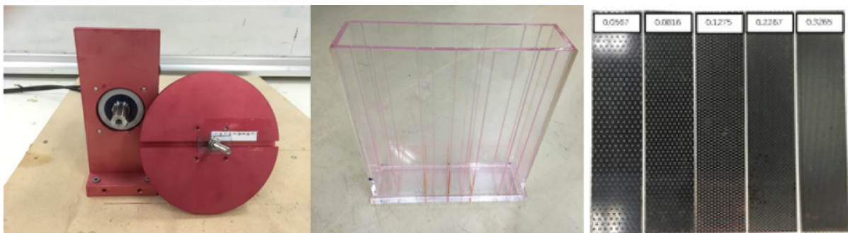
Fig. 2 Actuator, rectangular tank, and porous baffles used in model test
