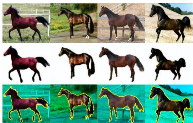
Fig. 8. Examples of representative segmentation results on the Weizmann horse dataset. From top to down: input images, results reported in [27], and our results.
