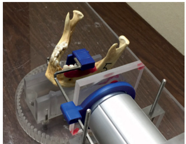
Fig. 1. A photograph shows the use of soft tissue simulation in acquiring intraoral radiographs.
