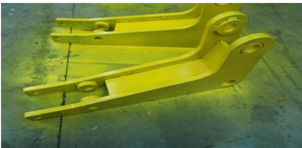
Fig. 11 Image of magnetic arm unit composed of 2 side plates and 1 rib plate used to connect the hydraulic cylinders
