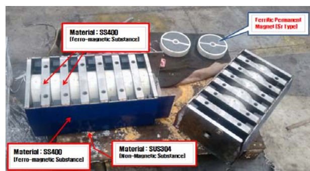
Fig. 9 Image to show the relationship between the individual components and the relevant materials used for the permanent magnet body
