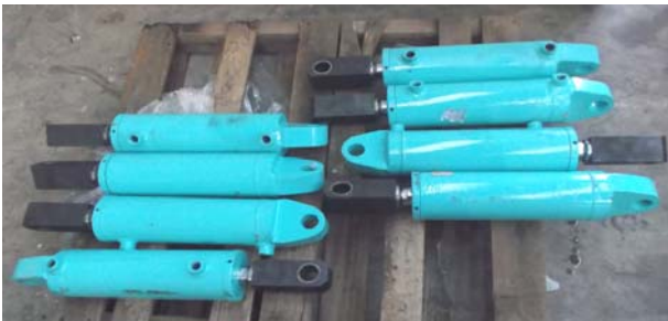
Fig. 10 Image to show the hydraulic cylinder used for the hydraulic, magnetic clamp device
