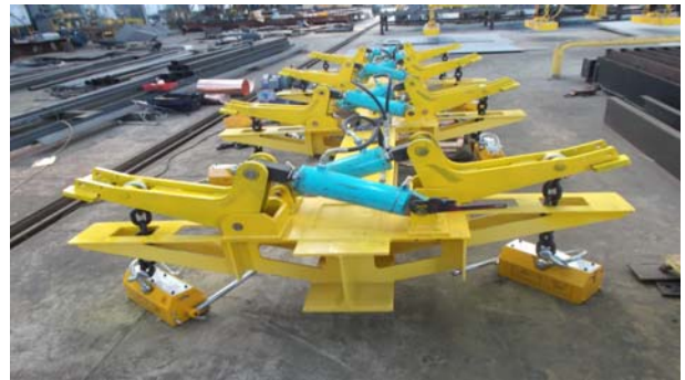
Fig. 12 Image of a assembled hydraulic-magnetic clamp
