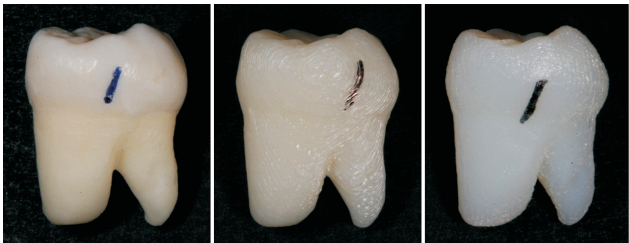
Figure 5. No. 1 original tooth (left) and replica teeth made with fused deposition modeling (middle) and PolyJet (right) three-dimensional printing technologies.
