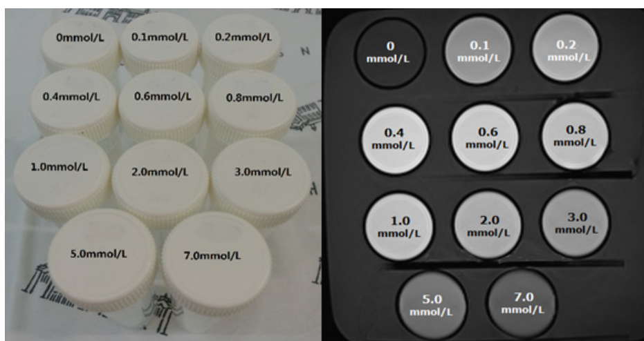
(left) The figure of agarose gel 2% contrast agent phantom, (right) fast spin echo T1 weighted image. The signal intensity was changed as a functional of molarity of gadoxetic acid.
