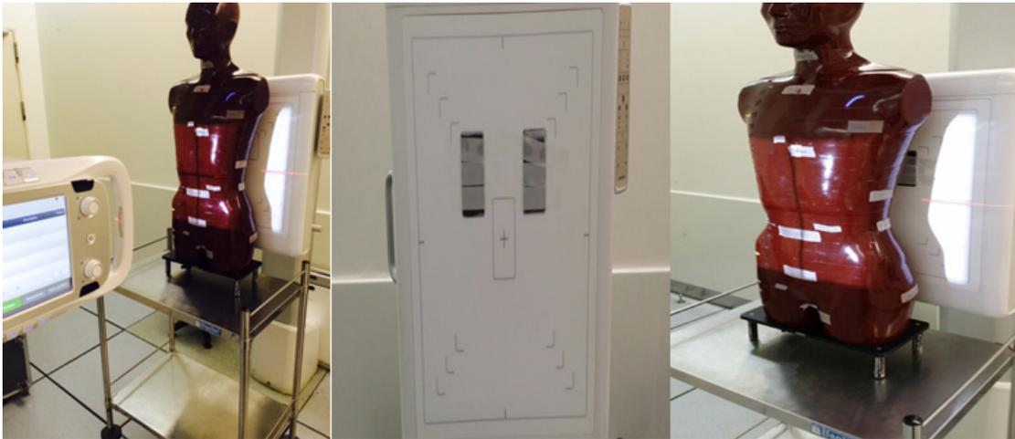
Figure 1 Acquiring images of abdomen AP in AEC mode with and without an attached metal on the ion chamber
