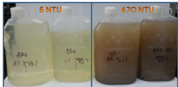
Fig. 5 Comparison of turbidity with respect to tillage method (left NT, right CT)
