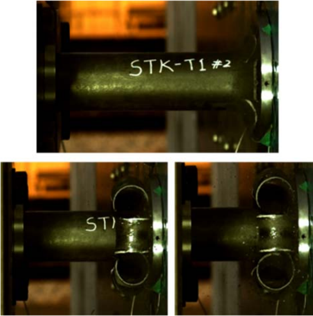
Fig. 5 Tearing tube curl deformation behavior on stage 1(top), stage 2(bottom left) and stage 3(bottom right)
