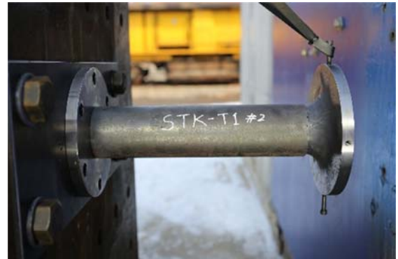
Fig. 11 Front view of collision test set-up
