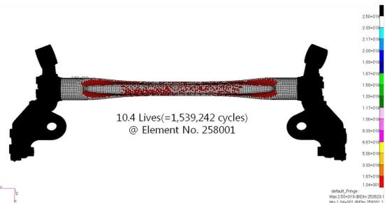
Fig. 10 Fatigue analysis result using MSC.Fatigue
