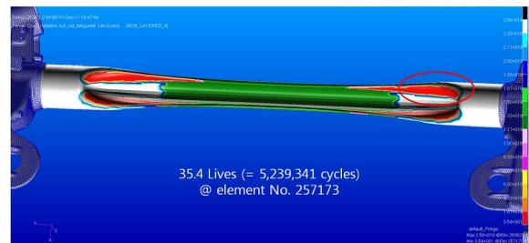
Fig. 11 Fatigue analysis result using ADAMS/Durability
