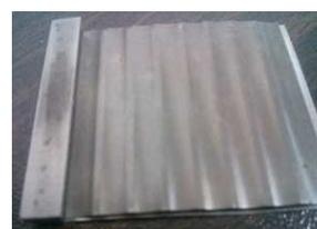
**Fig. 3** Photo of test GFB (left) and geometry of bump structure (right)
