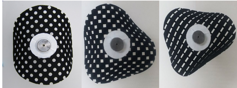
c8 S7 R12 Figure 5. Shape of Drapes of Motifs with Same Area
