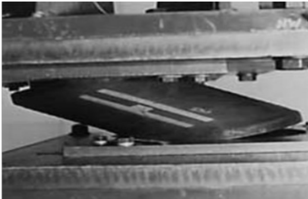
(a) Isolator Failure due to Large Deformation
