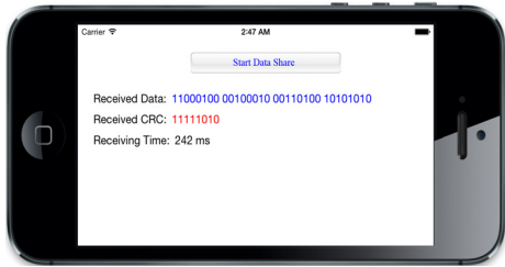
Fig. 5. Screen Shot of the Application which Receives Wireless Data
