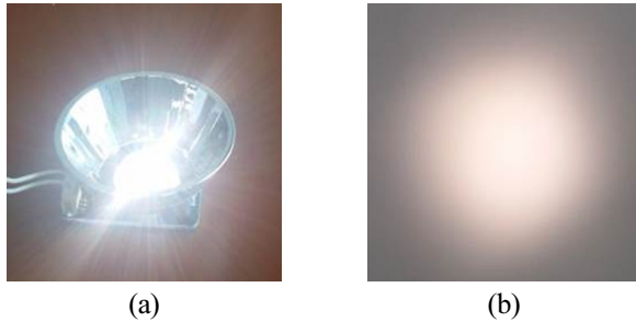
FIG. 10. Output beam based on the operation of single optical system: (a) Operation of single optical system (b) Output beam pattern on the white wall.
