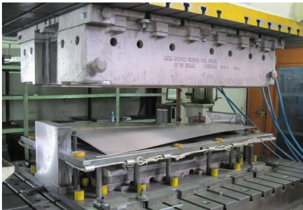
Fig.18 Dash panel blank before drawing
