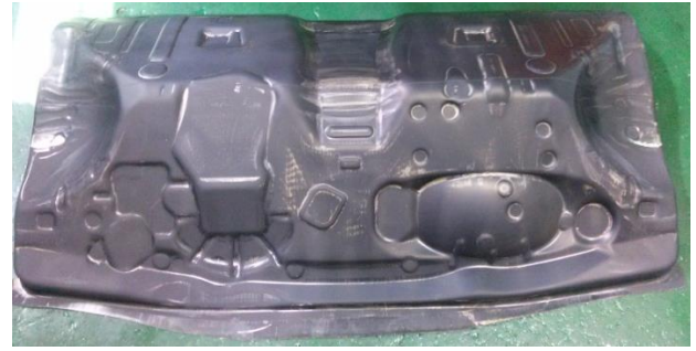
Fig.20 Drawing part of dash panel(thickness 2mm)
