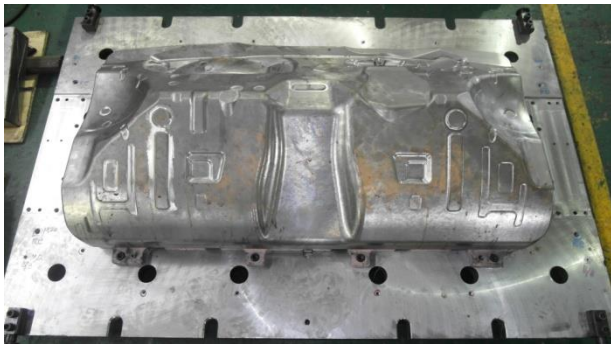
Fig.15 Lower shoe of dash panel mold
