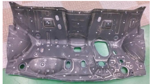
Fig.21 Final dash panel product(thickness 2mm)
