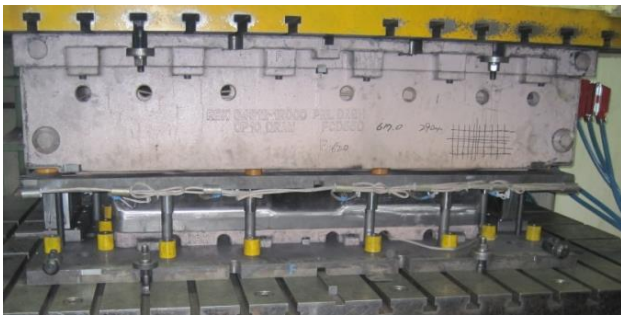
Fig.16 Dash panel mold before drawing
