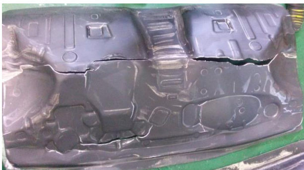
Fig.19 Drawing part of dash panel(thickness 1mm)
