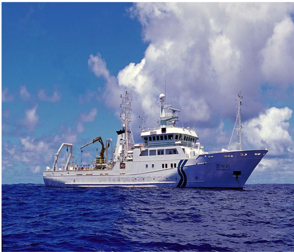
Fig. 2. Photograph of R/V Onnuri in KIOST (Length Over All: 63.8 m, Width: 12.0 m, Gross tonnage: 1,422 ton)
