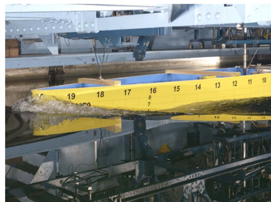
Fig. 7. Resistance test using scaled model ship (left: 12 knots, right: 15 knots)
