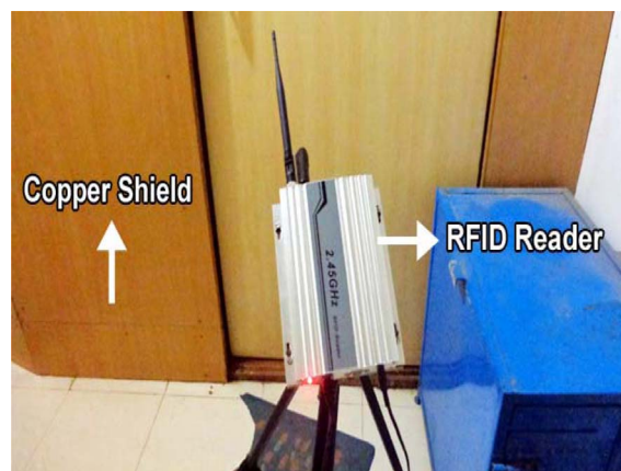
Fig. 4. (Color online) RFID reader positioned at 45° angle.
