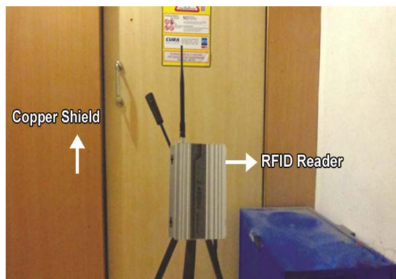
Fig. 3. (Color online) RFID reader positioned at 0° angle.
