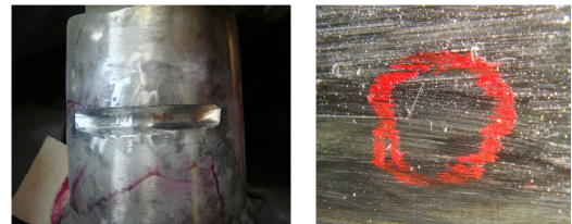
Fig. 13 Photo of porosity in mockup
