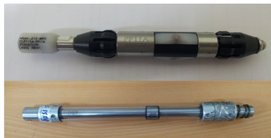
Fig. 12 Rotating probe and EDM-notch calibration standard
