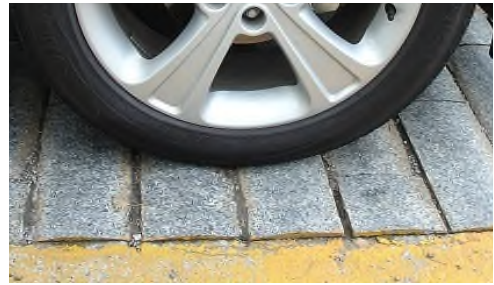
Fig. 1 Vehicle tests on the actual rattle road
