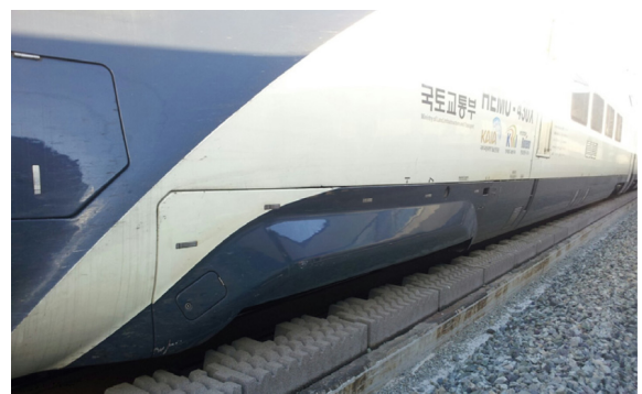
Fig. 3. Attachment of bogie fairing.
