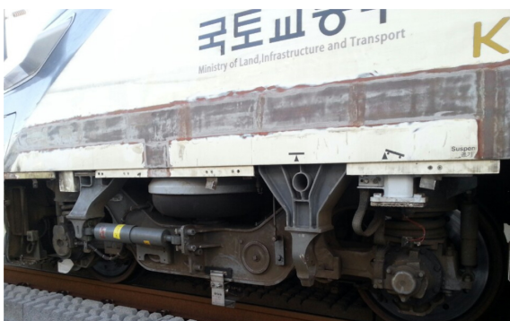
Fig. 2. Detachment of bogie fairing.
