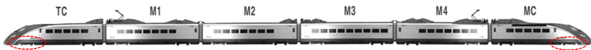
Fig. 1. Schematic picture of HEMU-430X train set and bogie fairing of nose car.
