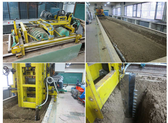
Figure 10. Soil preparation equipment (top left), prepared soil (top right), and RHSS attachment (bottom) for soil bin performance test.
