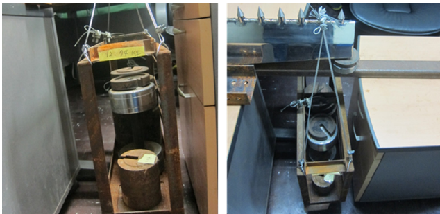
Figure 7. Testing view for calibration of RHSS sensor output.
