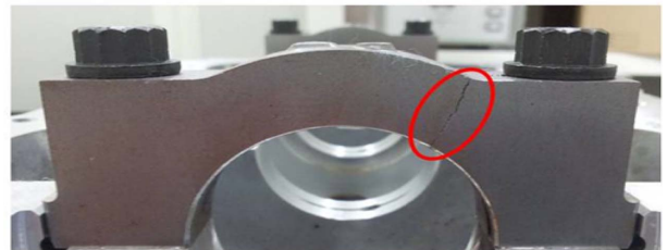
Fracture location Fig. 13. Location of Fatigue Fracture
