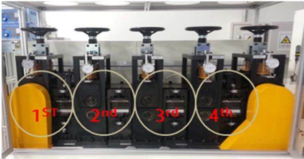
Fig. 6. 4 section of double belt laminator
