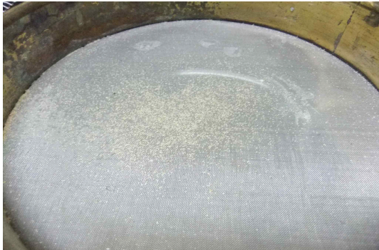
Fig. 4. Rice husk organic filler particles remaining on 60 mesh sieve.
