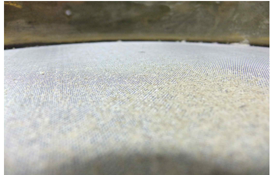
Fig. 4. Rice husk organic filler particles remaining on 60 mesh sieve.
