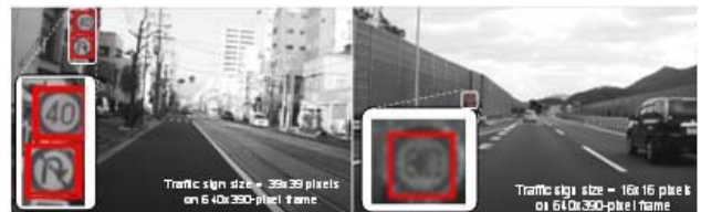
Fig. 20. Daytime scenes in local road and highway with sign distortion: recognizable with no difficulty.
