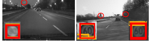
Fig. 23. German frames at day and night times in grayscale. Both are detectable and recognizable.
