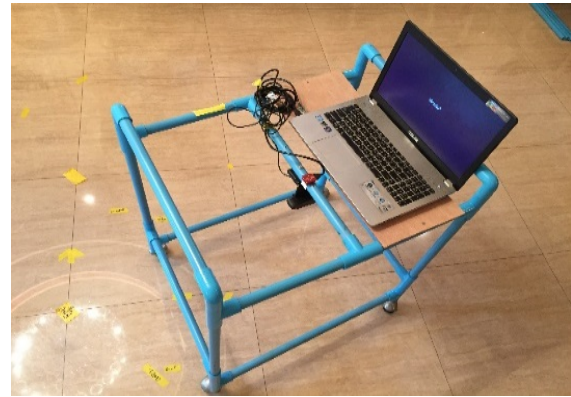
Fig. 2. Prototype frame for testing visual odometry.
