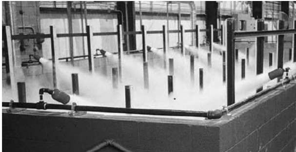
Figure 2. A discharge testing of carbon dioxide systems.
