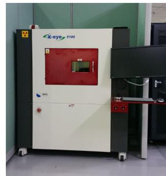
Fig. 1. Schematic diagram (a) and system (b) for imaging electronic components.
