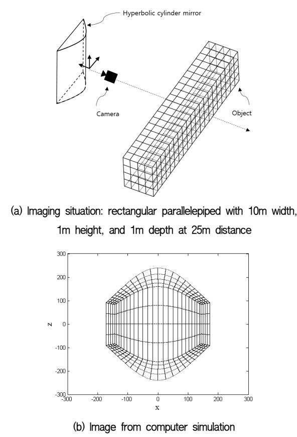
Fig. 5. Computer simulation for image acquisition model
