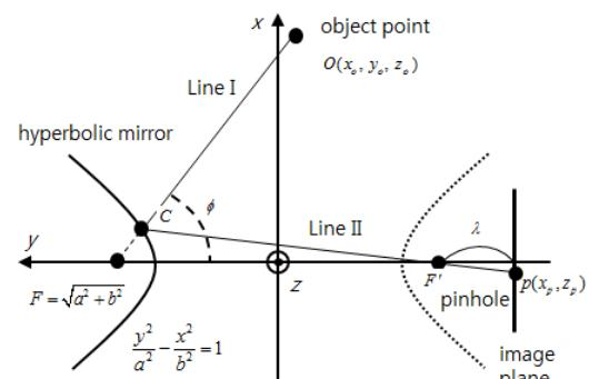
Fig. 2. Image acquisition model in horizontal  $x-y$  plane
