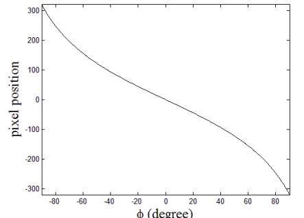
Fig. 6. Horizontal angular resolution of image with cylinder hyperbolic mirror
