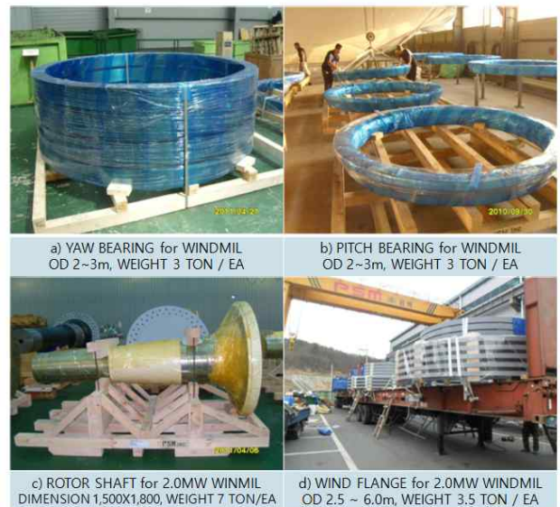
Fig. 3 Main equipments for wind power energy
