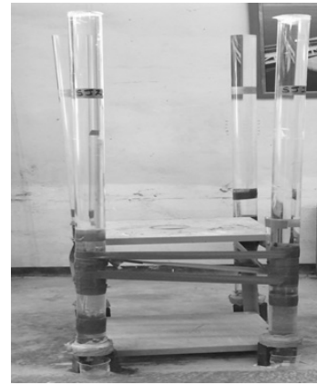
Fig. 3 Photo for water penetration test
