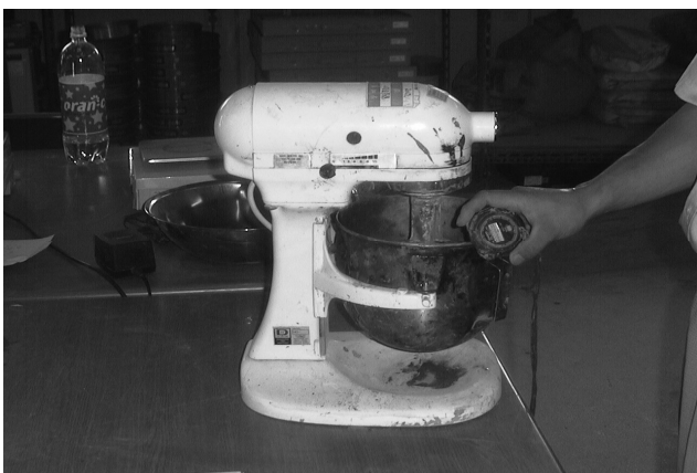
Fig. 3 Hopper type mixer for SMW mixing
