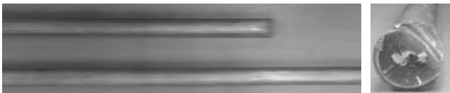
Fig. 12 Breakage shape of energy frame (Aluminium)
