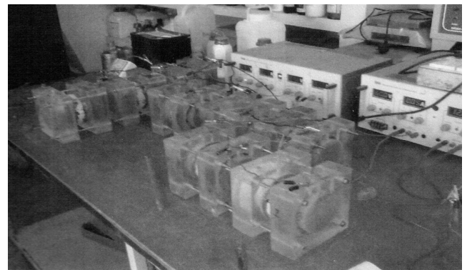
Fig. 2 Test setup for RCPT
