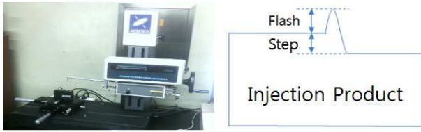
Fig. 4 Surface measuring machine and definition of the flash and step
