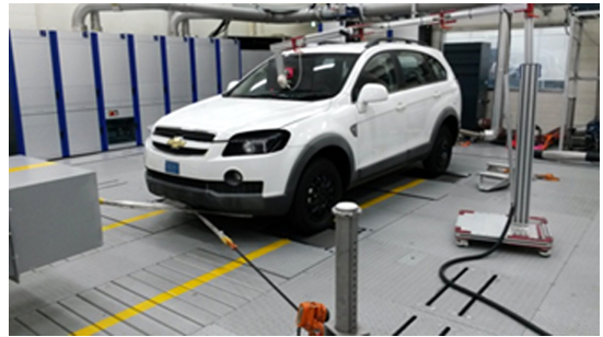
Fig. 4 Chassis dynamometer and exhaust measurement facility at Korea Automobile Testing & Research Institute
