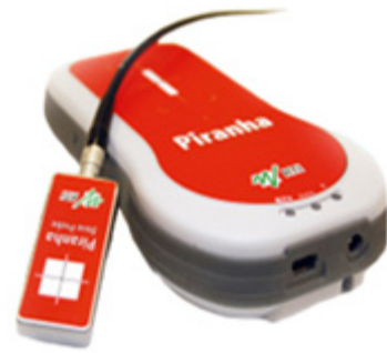
Figure 3 The Piranha 657 which is semiconductor dosimeter measuring the skin dose.
