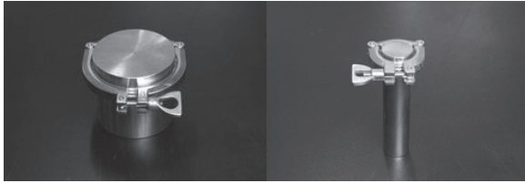
Fig. 1. Migration cells used for the tests (left: single-side contact cell, right: double-side contact cell)
