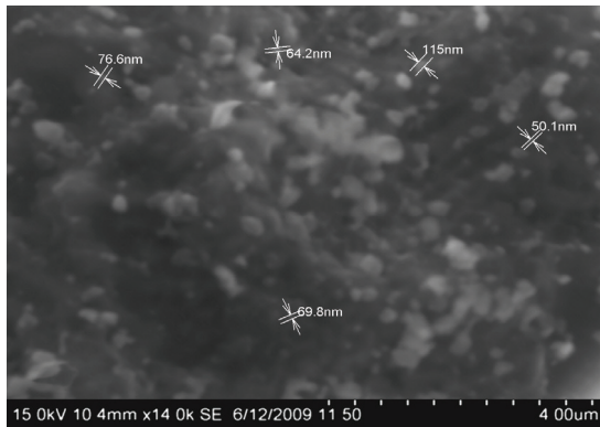
Fig. 2. SEM analysis of zirconia at 4\mu\text{m}
