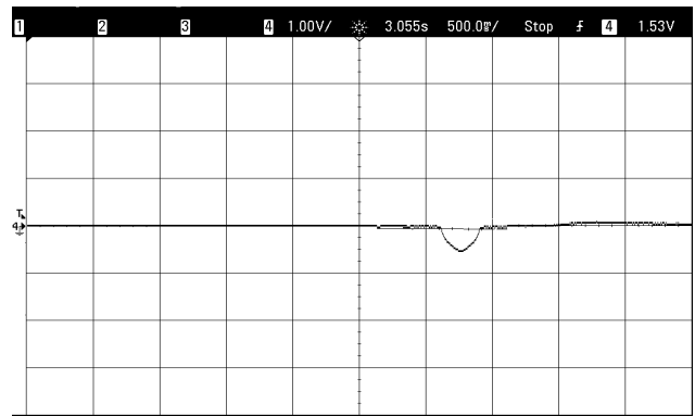
Fig. 16. Experimental dynamic response of DC-link voltage under step change load condition (load varies from 1KW to 1.5 KW)
