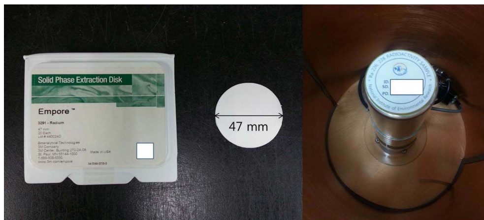
Fig. 1. Picture of the solid phase extraction disk and the analysing view for a pretreated disk.
