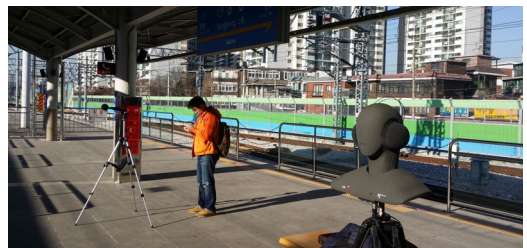
Fig. 1 Noise recording at station platform
