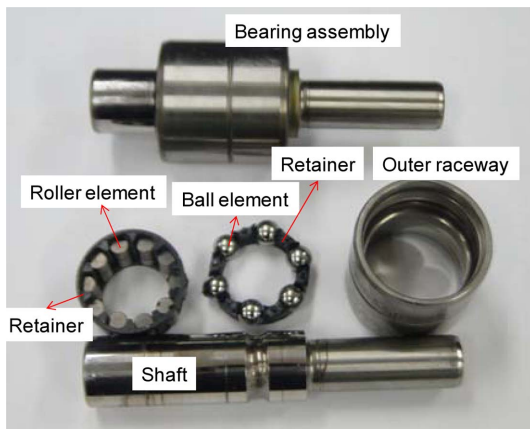
Fig. 1. General configuration of water-pump bearing.
