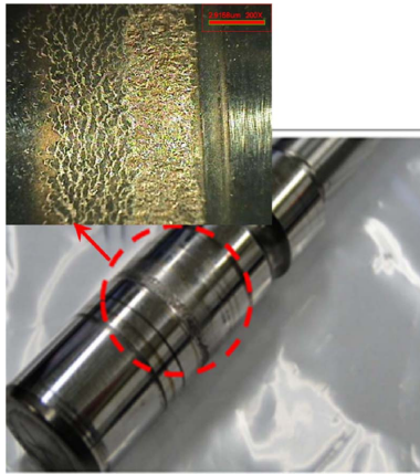
Fig. 11. Spalling of roller contact area.
