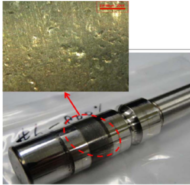
Fig. 7. Spalling of roller contact area (preliminary test).
