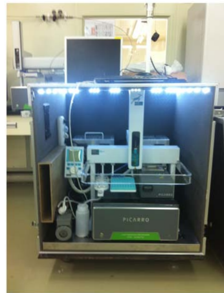
Fig. 2. Portable measurements of water vapor isotopes.
