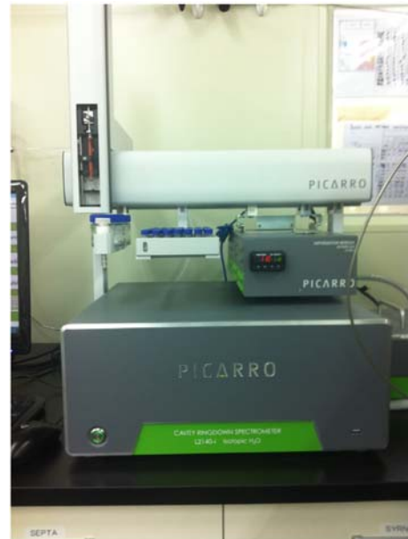
Fig. 1. Analyzer of stable water vapor isotopes (a new version, L2140).
