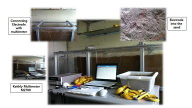
Fig. 3. Full set up of a sandbox experiment.
