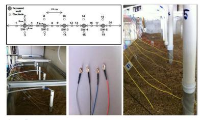
Fig. 4. Electrode set up into the sandbox.
