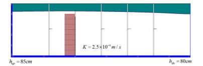
(a) Simulated water table with the injection rate of 0.005 L/sec
