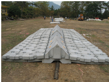
(c) AS-FCM (Anchor resistant Steel forced-FCM)
