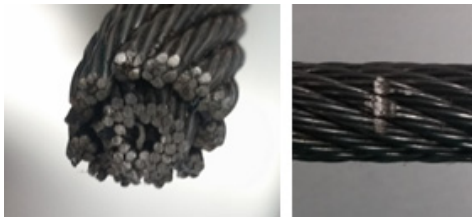
Fig. 15 Wire rope specimen & partial cutting damage
