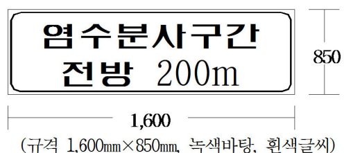
Fig. 3 Traffic Sign for Anti-icing Spray Roadway Section
